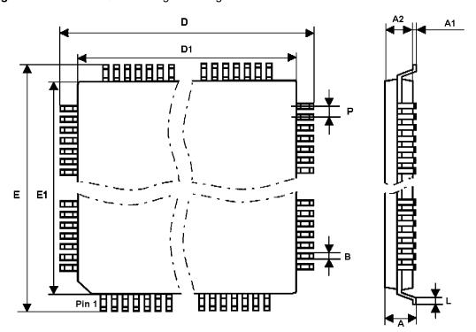
Table 9. 144-lead TQFP Package Dimensions (in millimeters)
