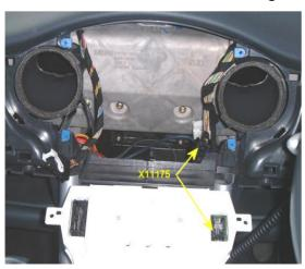
Remove the four screws on the corners of the Speedo. Now it should be free and you can tip it forward to reveal the two connectors.
