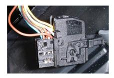
Remove the connector from the Speedo and then remove it from the housing.
