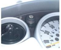
Now tug the panel sharply from the bottom on both sides to release it from the retaining clips. Now wiggle the panel off. This will now leave the Speedo exposed so be extremely careful not to damage it.
